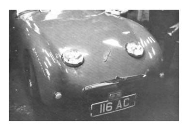
The two lamps were fixed onto hinges joined by a tube and activated mechanically so that they would swing up and forward to their operating position. When not in use, the lamps lay back flush with the bonnet. Unfortunately, in conjunction with the one-piece bonnet hinged at the back, this mechanism proved too complex and expensive, and was installed only on the first prototype. Porsche later used an almost identical pop-up headlamp system on their 928 model.
