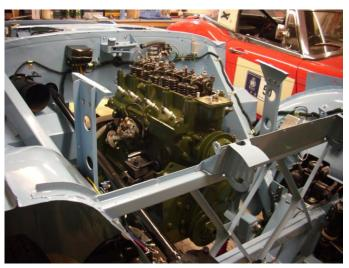
A completely new wiring loom is being fitted, I don't believe in taking chances with electrical stuff, and some of the instruments have been away for refurbishing. Rumour has it that there is no such thing as an accurate Healey fuel gauge, but at least we will have tried!
